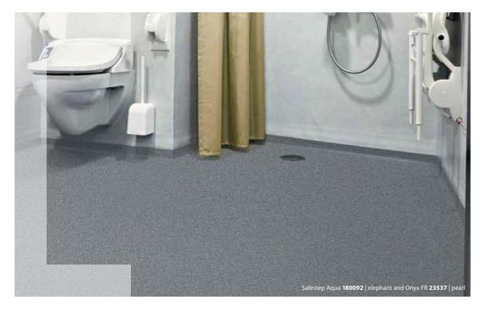
Onyx FR is a durable vinyl wallcovering, especially suited for wetrooms, such as bathrooms and showers. Once heat welded, it provides the perfect hygienic surface which ensures there is no breeding ground for bacteria. Matching weld rods are available.
